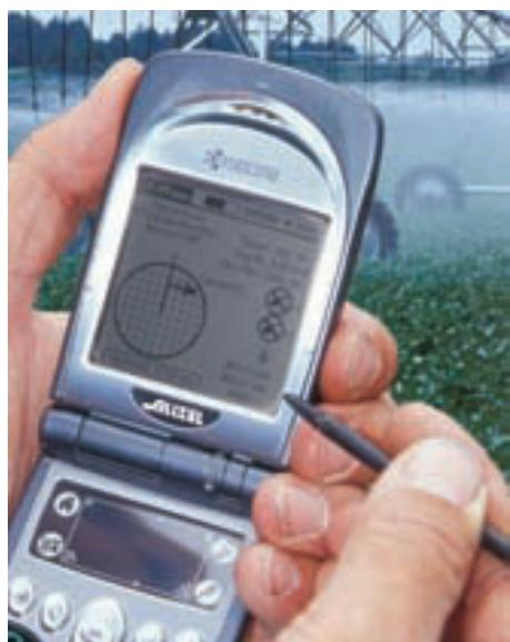
office sending the desired operations either by radio or wireless phones. Cell phones are already able to communicate with center pivots to monitor and control the operation status of the center pivot on a real time basis. It is also possible to use the internet to monitor and control an irrigation system. Using the internet a farmer will be able to control his irrigation system from anywhere in the world.
